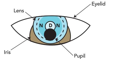
**Figure 21:** Spherical rotational design, lens translates up on down gaze
