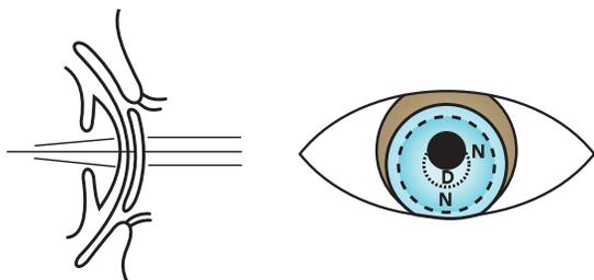
Figure 4a: Rotational design, looking straight ahead
