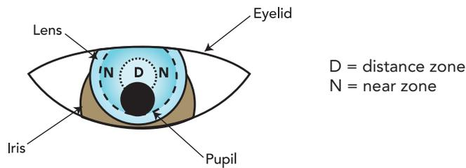
**Figure 20:** Aspheric rotational design, lens translates up on down gaze
