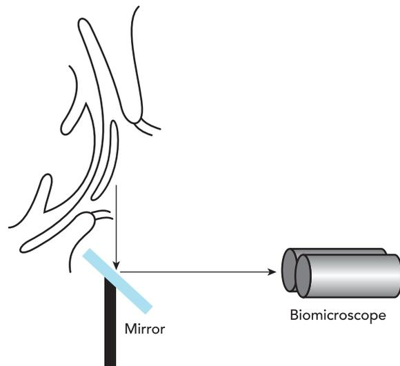
Figure 19b: Set-up to view lens in downward gaze
