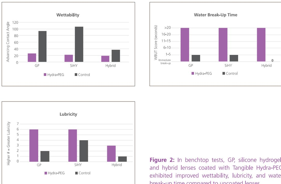
**Figure 2:** In benchtop tests, GP, silicone hydrogel, and hybrid lenses coated with Tangible Hydra-PEG exhibited improved wettability, lubricity, and water break-up time compared to uncoated lenses
